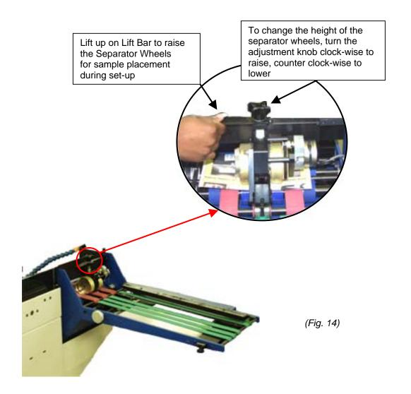
7. Adjust the height of the separator wheels by turning the adjustment knob (Clock-wise to raise, counter clockwise to lower) until light resistance is felt when pulling on the set up sample, see figure 14.
