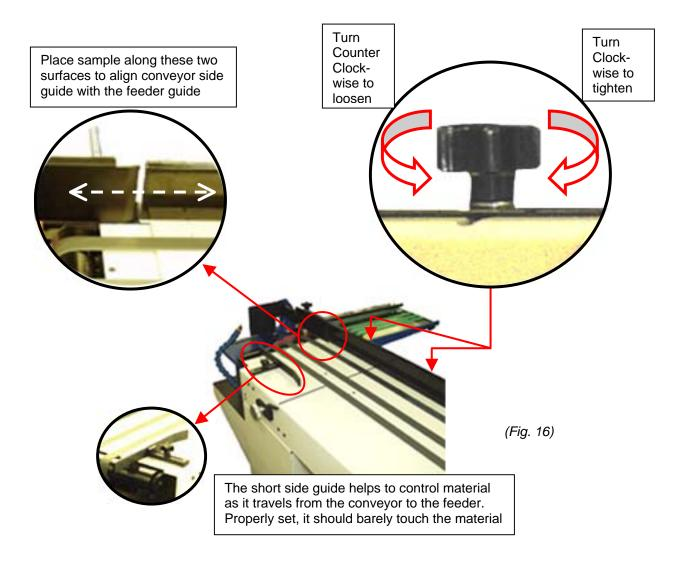
13. Once the exit roller of the in-feed conveyor has been extended and the in-feed conveyor long side guide has been set, manually draw the material from the top of the stack, placed in to the feeder in step # 10, onto the in-feed conveyor, see figure .
