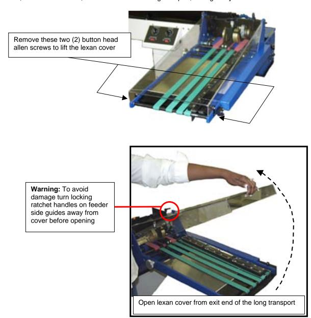
**Special Warning:** After the set-up is complete, be sure to re-secure the clear lexan cover to the exit end of the long transport using the button head screws previously removed in step # 6. The manufacture and other companies connected with the promotion and sale of the FeedMAX and FeedMAX-S do not recommend running the FeedMAX or FeedMAX-S with the clear lexan cover loose or removed.
