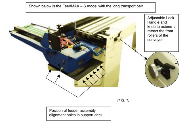
4. Using a philps head screwdriver, remove the paper guide located on the exit end of the in-feed conveyor, see figure. (Note: The paper guide is only used when running the Feed Max in a right angle configuration and must be removed before lifting the feeder up to re-position for straight in-line operation.) (Warning: Lifting the feeder with out removing the paper guide may result in damage to the machine as well as possible personal injury.)
