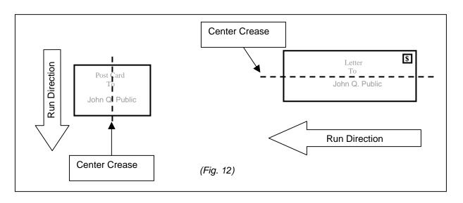
4. Set the creased sample in the feeder and align the crease with the philps head screws in the center of the stainless steel shroud of the separator wheels, see figure .
